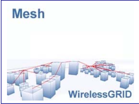
Figure 4. This diagram illustrates the combined use of WirelessGRID backhaul, repeater and multi-point equipment to cover a large geographic area, creating a mesh network.
